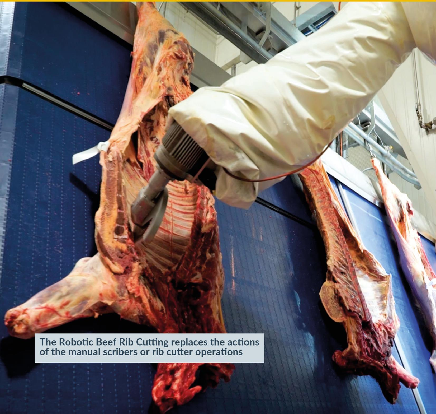
The Robotic Beef Rib Cutting replaces the actions of the manual scribes or rib cutter operations
